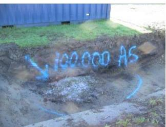
A quick XRF check revealed extreme copper, chromium & arsenic concentrations in some ashes.
